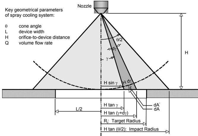
Optimum configuration (impact radius equal to device width):  $L/2 = H \tan(\theta/2)$
