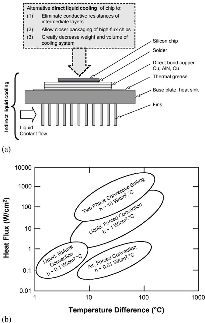
**Fig. 2** (a) Cooling path for removing heat from silicon die using indirect cooling with water/ethylene glycol, and alternative direct liquid cooling; (b) capabilities of existing cooling technologies using various fluids and operating pressures.
